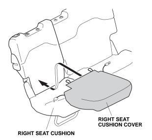
15. Lift up the right seat cushion. Secure the right seat cushion cover to the right seat cushion with two hooks and two loops.
