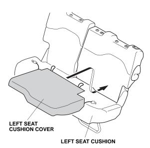
8. Lift up the left seat cushion. Secure the left seat cushion cover to the left seat cushion with two hooks and two loops.
