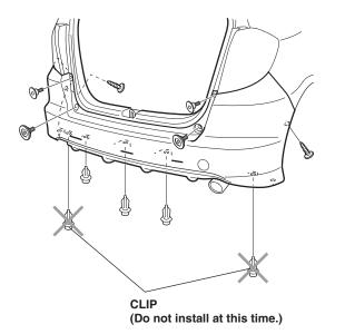
18. With the help of an assistant, place the rear under spoiler on the rear bumper. Bring the edge of the rear under spoiler up to the white marks made in step 4, and align the cutout in the under spoiler with the tow hook access cover.
