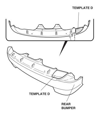
10. Using an airsaw, cut the rear bumper along the line. Use a file to remove any burrs from the edge.
