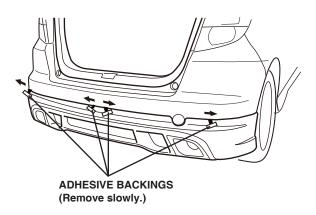
21. Using the palm of your hand, hold the spoiler firmly against the bumper for 30 seconds. Using a rubber roller, apply firm pressure while rolling to set the adhesive.
