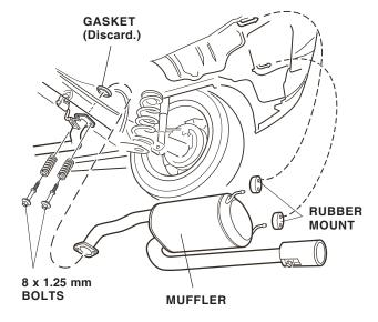
Remove and discard the old exhaust gasket, and install the new gasket from the kit.
