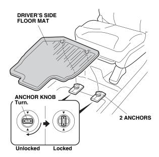
2. Turn the knobs on the anchors to secure the driver's side floor mat.
