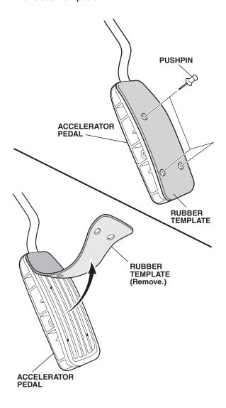
3. Place a block of wood under the accelerator pedal for support. While wearing eye protection, hold the accelerator pedal against the wood block and drill a 3 mm hole at each pierced mark. Wrap electrical tape around the drill bit 7 mm from the tip so you drill through only the first layer of the pedal.
