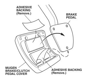
10. Remove the adhesive backing from the Mugen brake pedal cover. Align the top of the brake pedal cover over the brake pedal as shown, and press the pedal cover into position.
