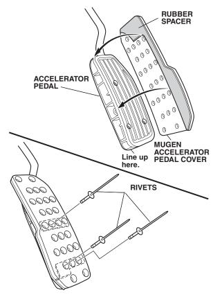
7. Place one spacer on each rivet. Using the rivet tool, compress each rivet while holding the spacer tight against the pedal. Remove the spacers.
