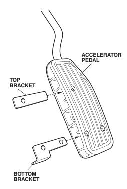
6. Place the Mugen accelerator pedal cover on the accelerator pedal with the top edge and the side edge of the rubber spacer tight against the pedal. Insert the three rivets through the pedal, the brackets, and the pedal cover at the holes shown.
