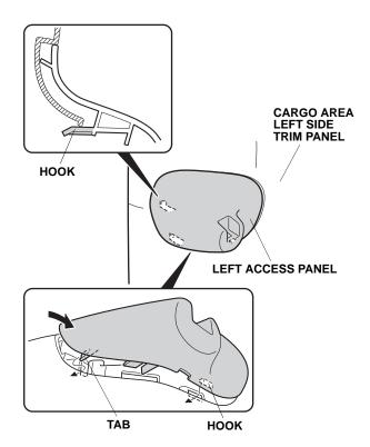
Push the left access panel in the direction shown to lock three tabs.
