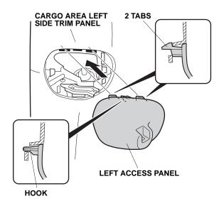
Insert one tab, and install two hooks.
