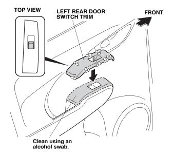
8. Attach the left rear door switch trim to the door switch panel as shown.
