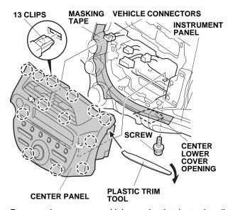
Remove the one screw. Using a plastic trim tool, pull the center panel out toward you to release the 13 clips. Unplug the vehicle connectors to remove the center panel.
