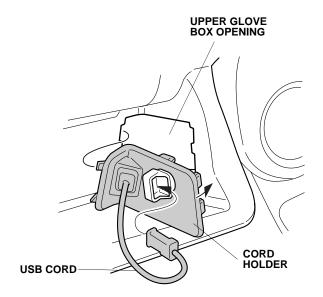
With the center panel near the dashboard, plug the USB cord connector into the control unit. Plug in all the vehicle connectors and reinstall the center panel.
