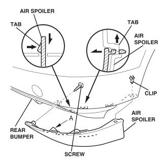
4. Place template A at three places on the rear bumper as shown, and mark the height of the rear under spoiler with a white marker on pieces of masking tape.
