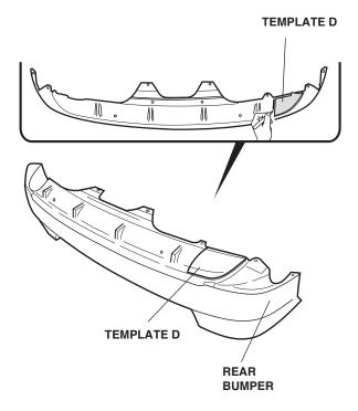
Using an airsaw, cut the rear bumper along the mark. Use a file to remove any burrs from the edge.
