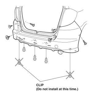
14. Using isopropyl alcohol on a shop towel, clean the rear bumper where the under spoiler will attach. Do not erase the white marks made in step 4. Allow the alcohol to dry.
