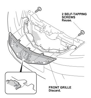
4. Using a utility knife, cut 5 mm from the top of the two center lock tabs as shown. If you do not cut the center lock tabs, the bumper cannot be removed because the tabs cannot release.
