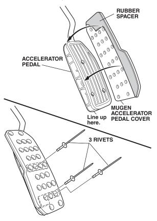
6. Place one spacer on each rivet. Using the rivet tool, compress each rivet while holding the spacer tight against the pedal. Remove the spacers.
