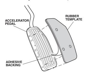
2. Using a pushpin, pierce the accelerator pedal at the center of each hole in the rubber template. Remove the rubber template.
