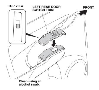
8. Attach the left rear door switch trim to the door switch shown.
