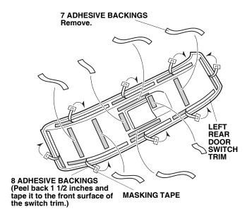
Clean the surface where the left rear door switch trim will be installed with an alcohol swab.
