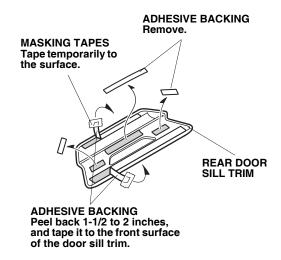
11. Clean the surface where the rear door sill trim will be installed using an alcohol swab.
