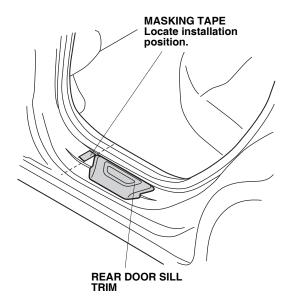
9. Align the rear door sill trim with the left door sill to check the installation location of the trim. Mark the location with a piece of masking tape.
