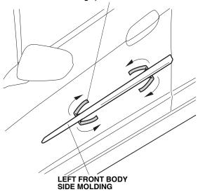
7. Using the rubber roller, apply firm pressure while rolling to set the adhesive.
