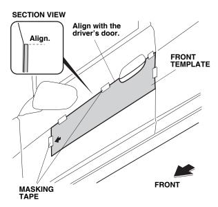
Peel back approximately 1 1/2 to 2 inches of adhesive backing from each adhesive tape, and tape the ends to the front surface of the body side molding. remove the small end pieces of the adhesive backing.
