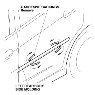
14. Using the rubber roller, apply firm pressure while rolling to set the adhesive.
