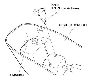
12. While wearing eye protection, drill the two pierced marks on the sides of the center console to 20 mm. First drill with a 3 mm drill bit, and finish with a 20 mm hole saw. Remove any burrs from the edges of the holes with a file.
