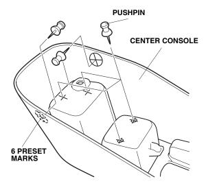
11. While wearing eye protection, drill the four pierced marks on the inside of the center console to 8 mm. First drill with a 3 mm drill bit, and finish with an 8 mm drill bit. Remove any burrs from the edges of the holes with a file.
