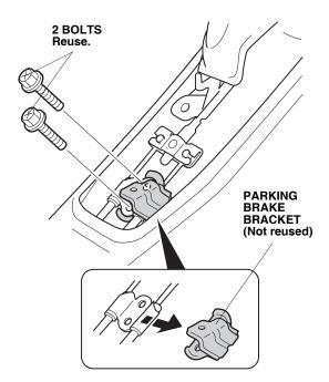
9. Install the floor bracket under the parking brake cables and reinstall the two bolts. Torque the bolts to 22 N·m (2.2 kgf·m, 16 lbf·ft).
