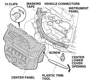
9. Remove the one screw. Using a plastic trim tool, pull the center panel out toward you to release the 13 clips. Unplug the vehicle connectors to remove the center panel.
