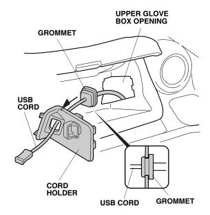
19. Install the cord holder into the upper glove box in place of the side cover and insert the end of the USB cord into the cord holder.
