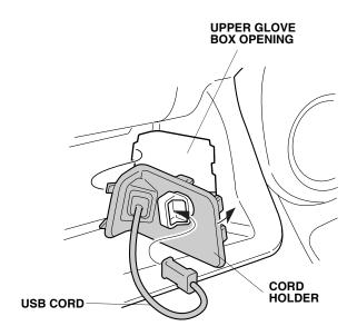
With the center panel near the dashboard, plug the USB cord connector into the control unit. Plug in all the vehicle connectors and reinstall the center panel.
