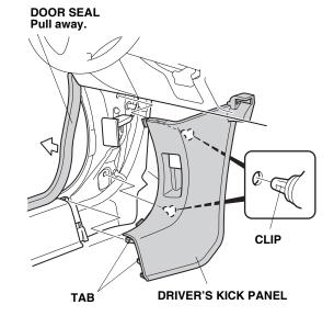
5. Remove the fuse access panel (five tabs, two clips and two hooks).
