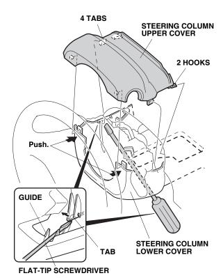
7. Remove the steering column upper cover (four tabs and two hooks).
