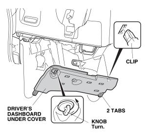
Pull away the door seal from the driver's kick panel, then remove the driver's kick panel (two clips and two tabs).
