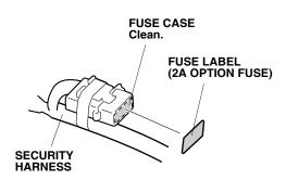
11. Attach the fuse label (2A OPTION FUSE) to the security system harness fuse case.
