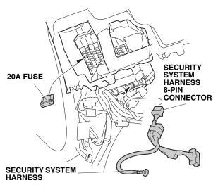
13. Install the 20A fuse to the fuse box in the location shown.
