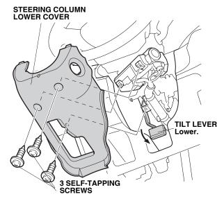
9. On the bottom of the steering column lower cover, cut off the small piece of the cover using a utility knife. Remove any burrs with a file.
