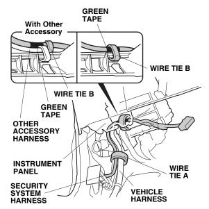
18. Using one wire tie B, secure the security system harness to the instrument panel as shown.
