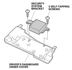
Plug the security system harness 18-pin connector to the control unit. Reinstall the driver's dashboard under cover.
