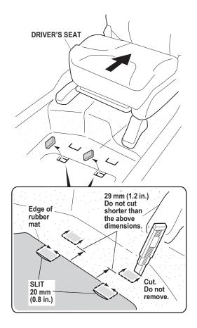
3. Locate the two recesses in the carpet. Using a utility knife, slit the carpet at the front of the recess. Do not cut out the piece between the recess and the rubber mat.
