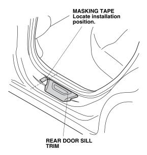
Align the rear door sill trim with the left door sill to check the installation location of the trim. Mark the location with a piece of masking tape. 10. Peel back approximately 1½ to 2 inches of adhesive backing of each outer adhesive tape, and tape the ends to the front surface of the rear door sill trim. Remove the remaining pieces of the adhesive backing from the trim.
