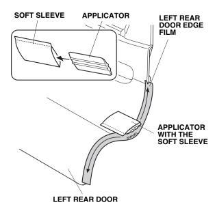
15. When your satisfied that the door edge film is firmly attached to the edge of the door, slowly remove the outer protective film.
