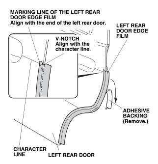
13. Continue to remove the adhesive backing while you align the center line on the door edge film with the edge of the door.
