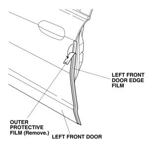
7. Starting in the middle of the door edge film and working outward, fold the left front door edge film around the door edge using your fingers. Move your finger in one direction. Attach the film over the seam sealant. Do not trim or damage the seam sealant.
