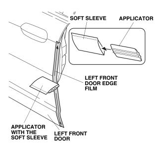
6. When your satisfied that the door film is firmly attached to the edge of the door, slowly remove the outer protective film.
