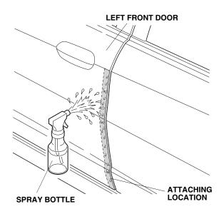
Open the left front door again. Peel back about 50 mm (2 in.) of adhesive backing from the left front door edge film. Align the V-notch in the door edge film with the end of the character line on the upper part of the front door.
