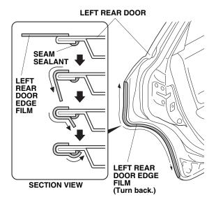
17. Using a lint-free shop towel, wipe up water from the rear door edge film. Allow the rear door edge film to dry thoroughly.
