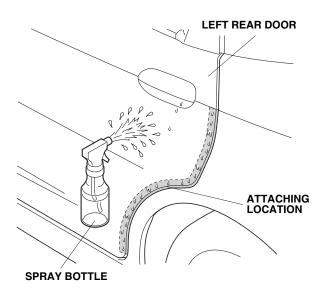
12. Open the left rear door again. Peel back about 50 mm (2 in.) of adhesive backing from the left rear door edge film. Align the V-notch in the door edge film with the end of the character line on the upper part of the left rear door.
