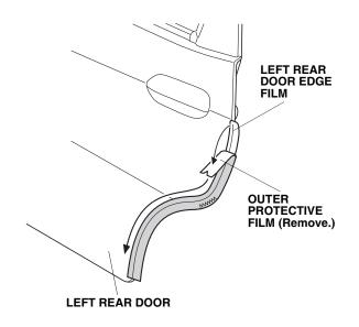
16. Starting in the middle of the door edge film and working outward, fold the door film around the door edge using your fingers. Move your finger in one direction. Attach the film over the seam sealant. Do not trim or damage the seam sealant.
