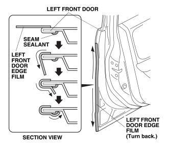
8. Using a lint-free shop towel, wipe up water from the front door edge film. Allow the front door edge film to dry thoroughly.
