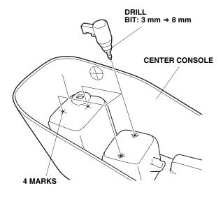
12. While wearing eye protection, drill the two pierced marks on the sides of the center console to 20 mm. First drill with a 3 mm drill bit, and finish with a 20 mm hole saw. Remove any burrs from the edge of the holes with a file.
