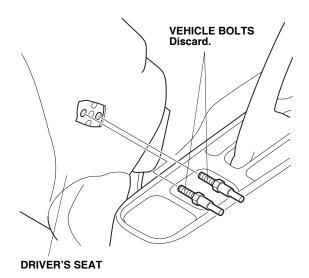
4. Place the new armrest cover over the seat and install the 10 x 30 mm washer bolt. Note the direction of the armrest cover. Install the new bolt cover over the bolt by engaging the back tab first.
