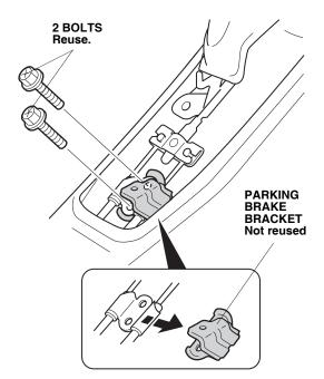
9. Install the floor bracket under the parking brake cables and reinstall the two bolts. Torque the bolts to 22 N·m (16 lb·ft). Be careful not to strip the threads.
