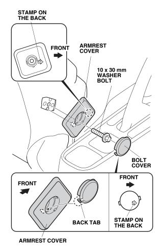
5. Remove the center console cover (three retaining tabs).
