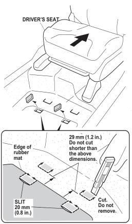
3. Locate the two recesses in the carpet. Using a utility knife, slit the carpet at the front of the recess. Do not cut out the piece between the recess and the rubber mat
