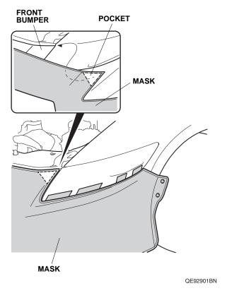
6. Pull the mask back toward the left front inner fender, smooth out any wrinkles, and secure two snaps on the mask to the two snap-screws.
