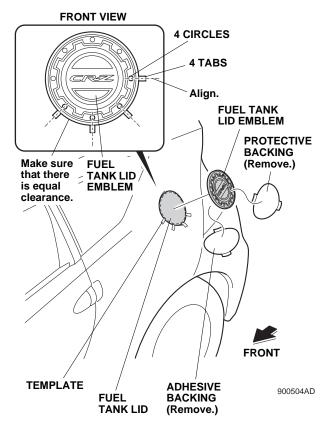
Line up the four circles on the fuel tank lid emblem with the four tabs on the template. Attach the fuel tank lid emblem to the fuel tank lid as shown. NOTE: Make sure that the fuel tank lid emblem is centered.
