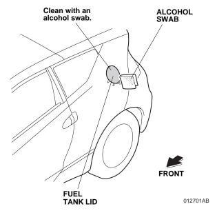
5. Using one alcohol swab, thoroughly clean the area where the fuel tank lid emblem will attach.
