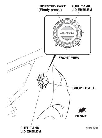
10. Using a shop towel, wipe the 3M protective tape application solution from the fuel tank lid and vehicle. Allow the fuel tank lid emblem to dry for 24 hours. NOTE: Do not open the fuel tank lid until the emblem is thoroughly dry.
