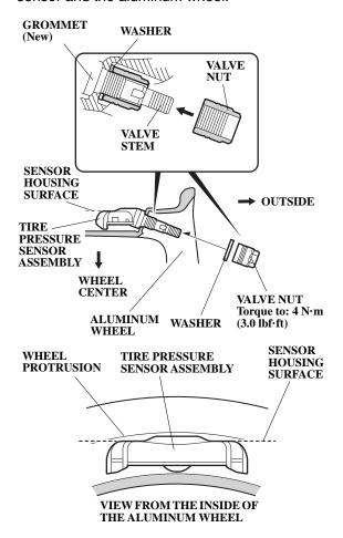
Install a new grommet, then install the tire pressure sensor and the washer to the wheel, and fingertighten the valve nut. Make sure the pressure sensor is resting on the wheel.
