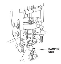
16. Compress the HPD damper spring.
