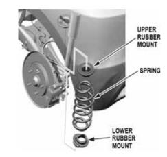
41. Install the upper rubber mount on the HPD rear spring by aligning the upper end of the rear spring with the ledge portion of the upper rubber mount.
