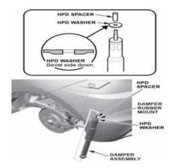
47. Slowly raise the jack until you can align the bolt hole with the holes in the axle beam and the damper, then loosely tighten the damper mounting bolt.
