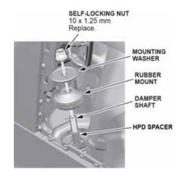
50. Torque the self-locking nut to 30 N•m (22 lb-ft) while holding the HPD damper shaft with an Allen wrench.
