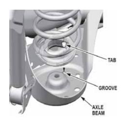
44. Position the floor jack under the lower spring seat on the axle beam.
