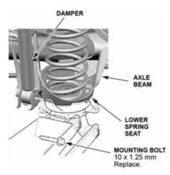
Raise the rear suspension with the jack until the vehicle just lifts off of the lift, then tighten the damper mounting bolts and torque to 54 N•m (40 lb-ft). 49. Install the damper rubber mount, the damper mounting washer, and the self-locking nut on the HPD damper shaft.
