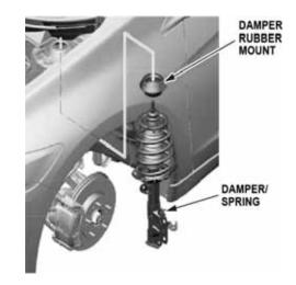
24. Install the damper mounting nut, the wave washer, and the mounting base.
