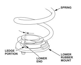
43. Install the tab of the lower rubber mount into the groove of the lower spring seat. NOTE: Make sure that the tab of the lower rubber mount is properly installed into the axle beam.
