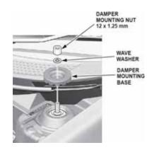
Remove the damper/spring assembly and the damper rubber mount.
