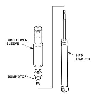
46. Install the HPD washer bevelside down, then the HPD spacer, and the damper rubber mount onto the HPD damper unit. Position the damper assembly between the body and the axle beam. NOTE: Be careful not to damage the body.
