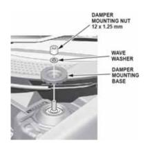
Hold the HPD damper shaft using an Allen wrench, and torque the damper mounting nut to 44 N•m (32 lb-ft).
