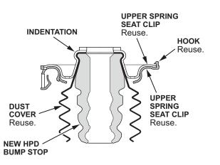
12. Install the HPD bump stop and the dust cover into the upper spring seat. Push the HPD bump stop and the dust cover into the indentation in the upper spring seat securely. 13. Install the HPD spring on the upper spring seat clip by aligning the upper end of the spring with the ledge portion of the upper spring seat clip.
