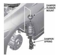
10. Using a strut spring compressor, compress the spring to relieve the tension on the upper spring seat, then remove the nut while holding the damper shaft with an Allen wrench.
