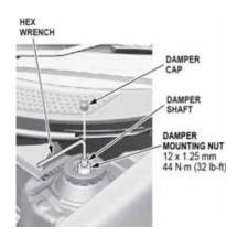
26. Install the damper cap to the top of the damper.
