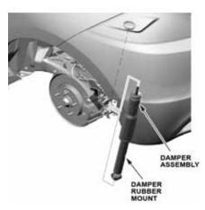
40. Lower the floor jack gradually. Remove the spring, the upper rubber mount, and the lower rubber mount.
