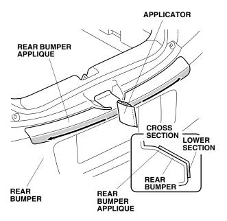
Using a shop towel, wipe the excess 3M protective tape application solution from the rear bumper applique. Allow the rear bumper applique to dry thoroughly.
