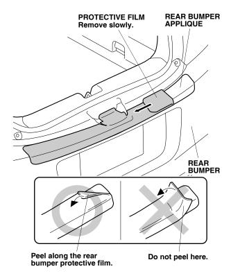
Once the flat surface is completely smooth with no bubbles, use the applicator with soft sleeve to apply the rear bumper applique to the rounded rear edge of the bumper.
