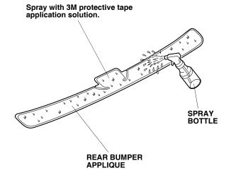
5. Align the edge of the rear bumper applique to the character line, and attach it to the rear bumper.
