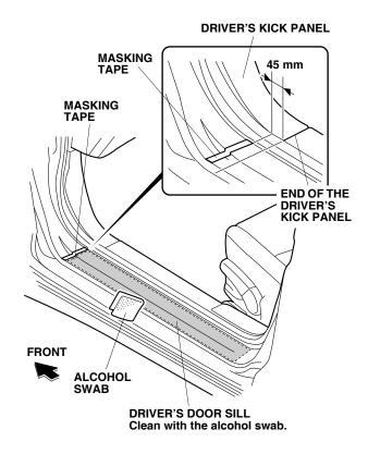
Using one alcohol swab, thoroughly clean the door sill where the driver's door sill trim will attach.
