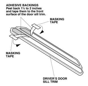
4. Align the front edge of the driver's door sill trim to the masking tape, and install the driver's door sill trim to the driver's door sill.
