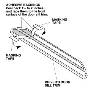
4. Align the front edge of the driver's door sill trim to the masking tape, and install the driver's door sill trim to the driver's door sill.
