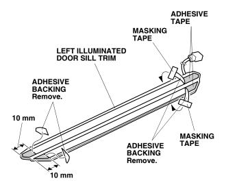
Using the alcohol swab, thoroughly clean the area where the left illuminated door sill trim will attach.
