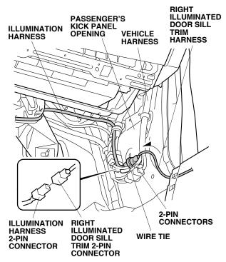
55. Secure the 2-pin connectors to the vehicle harness with one wire tie.
