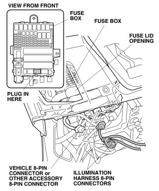
Plug the vehicle 8-pin connector or other accessory 8-pin connector into the illumination harness 8-pin connector.
