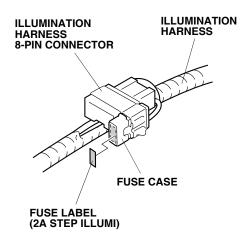
Unplug the vehicle 8-pin connector or other accessory 8-pin connector (if equipped) from the fuse box, and plug the illumination harness 8-pin connector into the fuse box.
