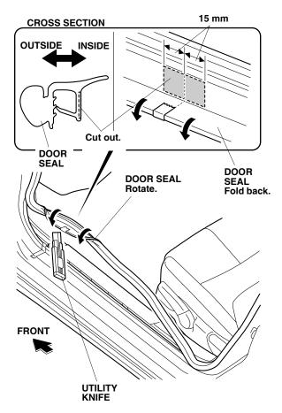
17. Using a utility knife, make a slit in the door seal rubber to expose the small metal plates inside the rubber seal.
