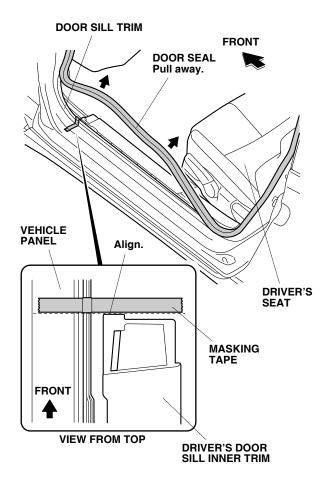
Attach a piece of masking tape to the vehicle panel even with the front edge of the driver's door sill inner trim.
