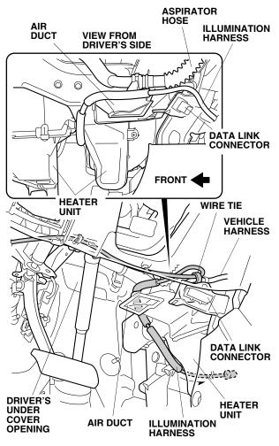
46. Secure the illumination harness to the vehicle harness with one wire tie.
