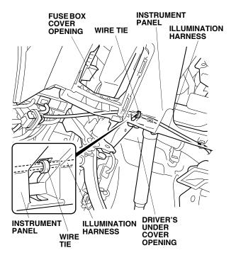
45. Route the illumination harness to the passenger side of the vehicle as shown.
