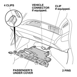
4. Pull away the door seal from around the passenger's kick panel, and remove the passenger's kick panel (two clips and three retaining tabs).
