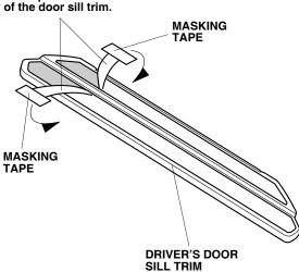
4. Align the front edge of the driver's door sill trim to the masking tape, and install the driver's door sill trim to the driver's door sill.
