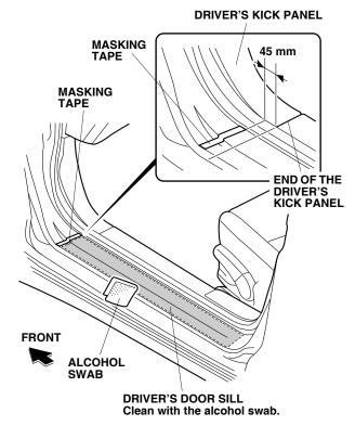
Using one alcohol swab, thoroughly clean the door 2. sill where the driver's door sill trim will attach.
