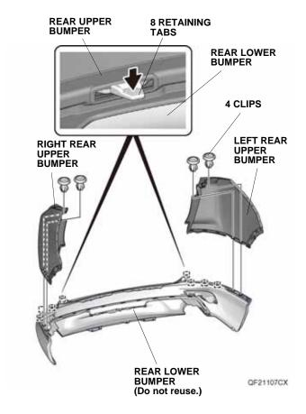
Install the left rear upper bumper to the rear aero bumper with two clips and four retaining tabs.
