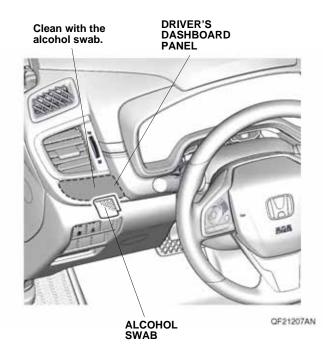
7. Peel back the adhesive backings, and tape them to the front surface of the driver's side panel with masking tape. Remove the remaining adhesive backing.
