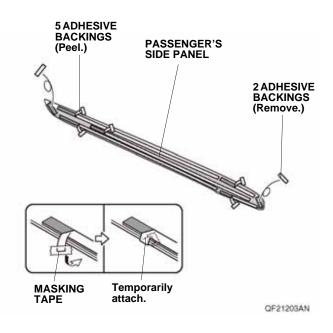
Attach the passenger's side panel to the passenger's dashboard trim panel as shown.
