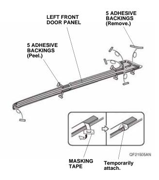
13. Line up and attach the left front door panel to the left front door as shown.
