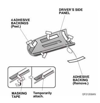
8. Attach the driver's side panel to the driver's dashboard panel as shown.
