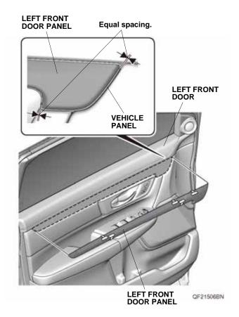
14. While applying light pressure against the left front door panel, carefully remove the taped adhesive backings.
