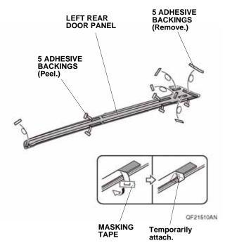
18. Line up and attach the left rear door panel to the left rear door as shown.
