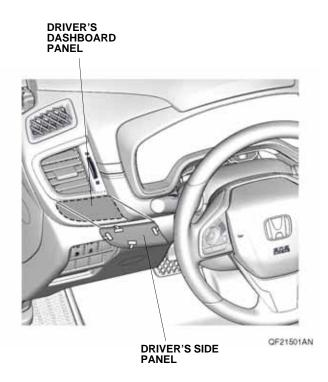
9. While applying light pressure against the driver's side panel, carefully remove the taped adhesive backings.
