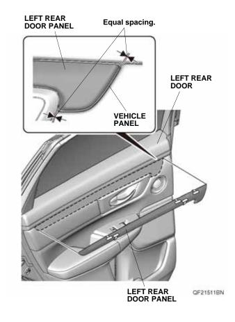
19. While applying light pressure against the left rear door panel, carefully remove the taped adhesive backings.
