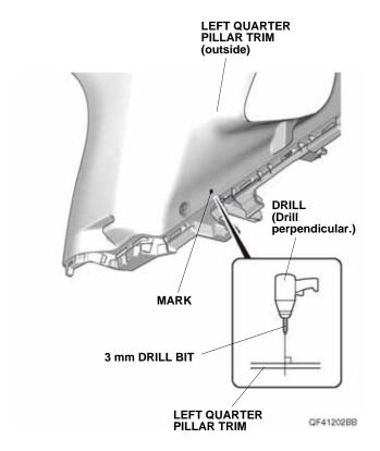
52. While wearing eye protection, enlarge the 3 mm hole to 26 mm using a 26 mm hole saw. Remove any burrs.
