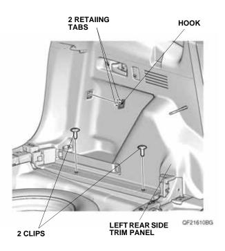
Pull away the door opening seal and weatherstrip from around the left rear side trim panel. Remove the left rear side trim panel, and unplug the vehicle connector.
