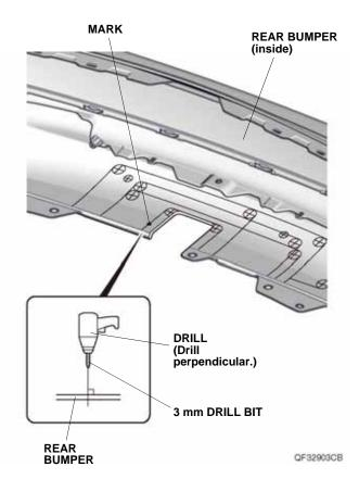
25. While wearing eye protection, enlarge the 3 mm hole to 14 mm using a 14 mm hole saw. Remove any burrs.
