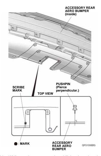
29. While wearing eye protection, drill the pierced mark on the accessory rear aero bumper with a 3 mm drill bit.
