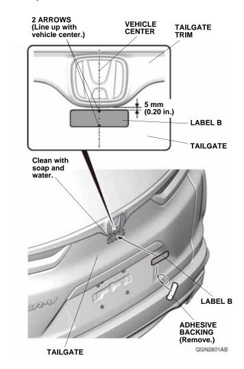
73. Remove the adhesive backing from the label B. Using the arrows on the label B, center it 5 mm (0.20 in.) below the tailgate trim and attach it to the tailgate.
