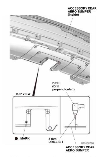
30. While wearing eye protection, enlarge the 3 mm hole to 14 mm using a 14 mm hole saw. Remove any burrs.
