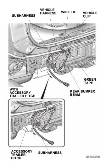
37. With the help of an assistant, bring the rear bumper close to the vehicle, and plug the subharness 3-pin
