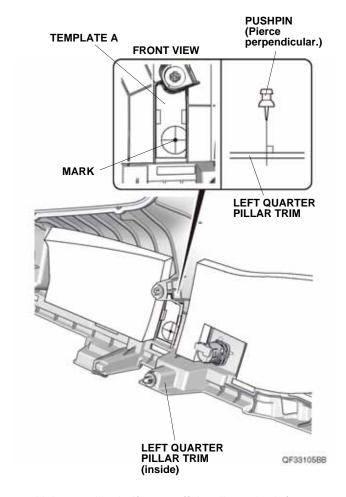
50. Using a utility knife, cut off the rib on the left quarter pillar trim as shown. Remove any burrs.
