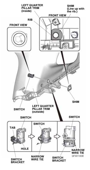
56. Line up the tab on the switch bracket with the hole on the switch, and secure the switch bracket to the switch with one narrow wire tie. Go to step 63. NOTE: Firmly press the switch bracket against the left quarter pillar trim, and make sure that there is no clearance between the switch and left quarter pillar trim.
