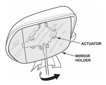
Insert a flat-tip screwdriver between the mirror holder and the actuator. Twist the screwdriver to release the hooks. 3. Remove the actuator from the new mirror holder.
