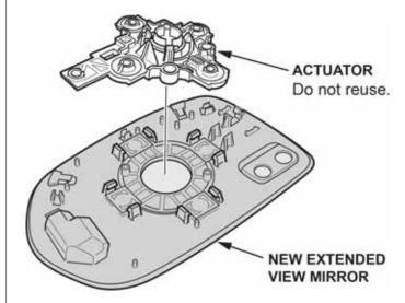
4. Line up the new mirror holder with the actuator and press in place.
