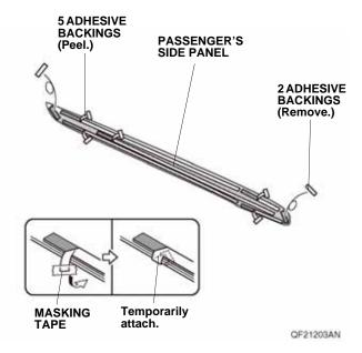
3. Attach the passenger's side panel to the passenger's dashboard trim panel as shown.
