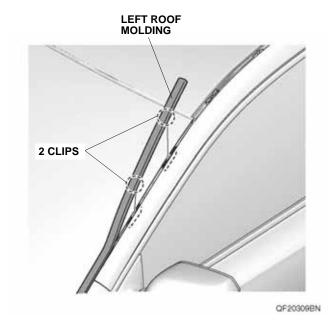
Insert two flat-tip screwdrivers alternately between four clips and four stud bolts as shown. While pulling on the clips, release the locking tabs on the clips from the groove on the stud bolts notch by notch, and remove the clips.
