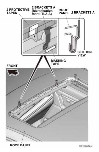
9. Set the moonroof visor on the roof in front of the moonroof opening, and adjust its position so the holes in the moonroof visor are lined up with the holes in brackets A. Loosely install the moonroof visor to brackets A with two screws and two nuts. Remove the strips of masking tape from brackets A.
