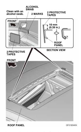
Remove the adhesive backing from the two protective tapes, and attach one to the roof panel at each of two marks you made. Wrap 10 mm (0.39 in.) of protective tape around the lip of the moonroof opening.  Locate the first indentations from the right front corner and left front corner of the moonroof opening. Using an alcohol swab, thoroughly clean the roof panel where the protective tapes will attach.
