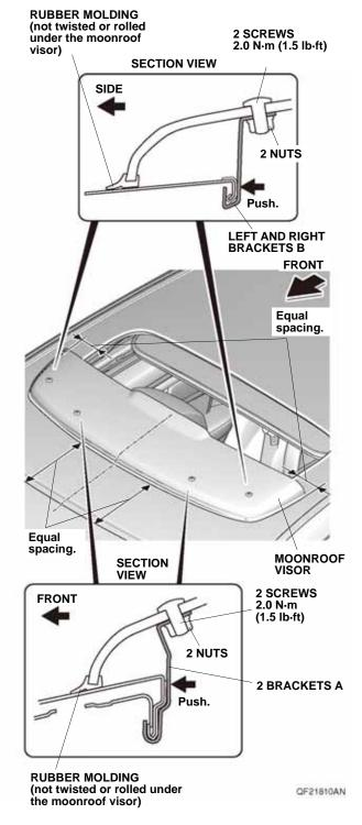
12. Tighten the two screws and two nuts on the front of the vehicle first, then tighten the two screws and two nuts on each side. Tighten while applying pressure so that there is no gap between the roof panel and brackets A and B. Torque the screws to 2.0 N·m (1.5 lb·ft).
