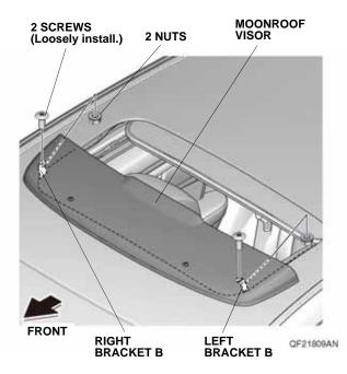
11. Position the moonroof visor with equal spacing on each side. Check that the rubber molding is not twisted or rolled under the moonroof visor.
