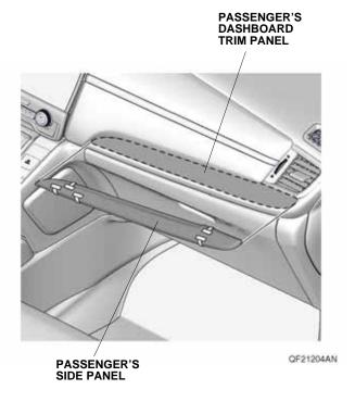
4. While applying light pressure against the passenger's side panel, carefully remove the taped adhesive backings.
