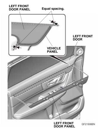
While applying light pressure against the left front door panel, carefully remove the taped adhesive backings.
