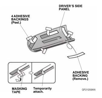
8. Attach the driver's side panel to the driver's dashboard panel as shown.
