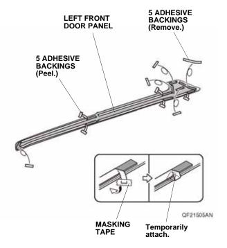
13. Line up and attach the left front door panel to the left front door as shown.
