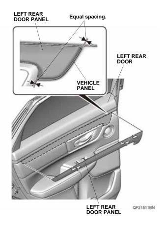
While applying light pressure against the left rear door panel, carefully remove the taped adhesive backings.
