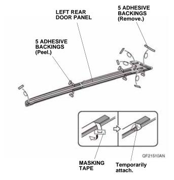
Line up and attach the left rear door panel to the left rear door as shown.
