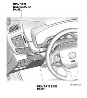
While applying light pressure against the driver's side panel, carefully remove the taped adhesive backings.
