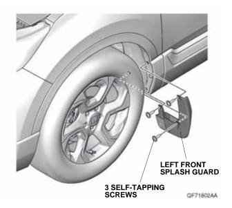
3. Remove the self-tapping screws, and clips from the left front wheel arch protector as shown.
