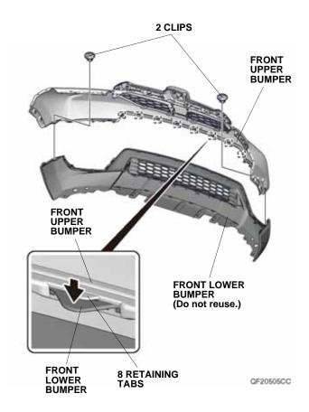
Install the front aero bumper to the front upper bumper with two clips and eight retaining tabs.
