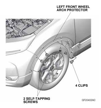
4. Remove the left front wheel arch protector as shown.
