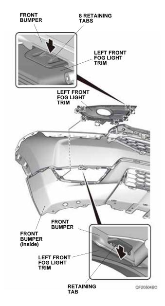
11. Remove the front lower bumper from the front upper bumper.
