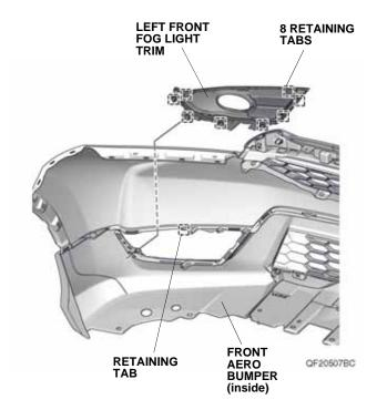
If the vehicle is equipped with halogen fog lights, continue with step 14; if the vehicle is equipped with LED fog lights, go to step 15; otherwise, go to step 16.
