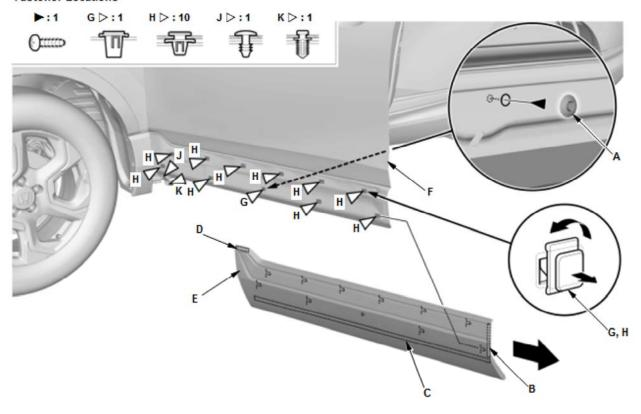
2. Cut the adhesive tape (B, C, D) along the edge of the door lower trim (E) with a utility knife while separating the trim from the door (F) with a trim tool.
