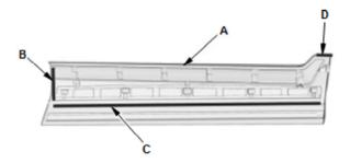
If you are reusing the original door lower trim (A), apply primer to the areas where new double-sided adhesive tapes (B, C, D) will be applied, then attach the new doublesided adhesive tapes to the trim as shown.
