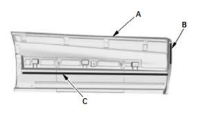
If you are reusing the original door lower trim (A), apply primer to the areas where new double-sided adhesive tapes (B, C) will be applied, then attach the new doublesided adhesive tapes to the trim as shown.
