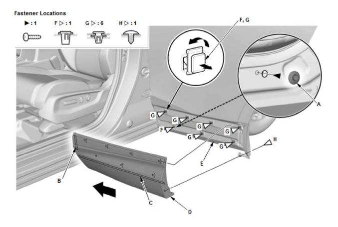
2. Cut the adhesive tape (B, C) along the edge of the door lower trim (D) with a utility knife while separating the trim from the door (E) with a trim tool.
