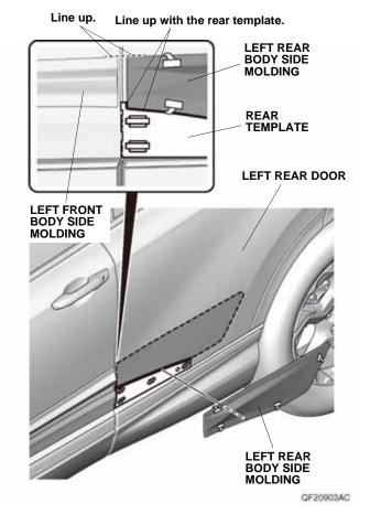
Make sure the edges of the left front body side molding and the left rear body side molding are lined up.
