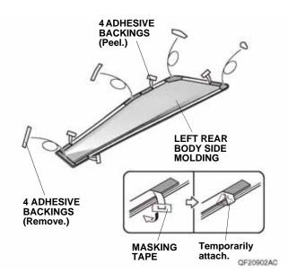
12. Line up the left rear body side molding with the rear template, and attach it to the left rear door as shown.
