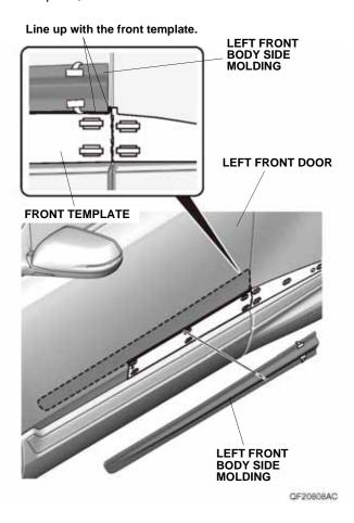
8. While applying light pressure against the left front body side molding, carefully remove the taped adhesive backings.
