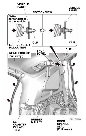
17. Using a rubber mallet wrapped with a shop towel, lightly tap the area marked "SIDE CURTAIN AIRBAG" on the left quarter pillar trim to push in the clip. Make sure to strike the area perpendicular to the vehicle.
