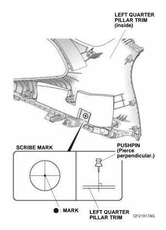
80. While wearing eye protection, drill the pierced mark on the left quarter pillar trim with a 3 mm drill bit. NOTE: Make sure to drill perpendicular to the left quarter pillar trim.
