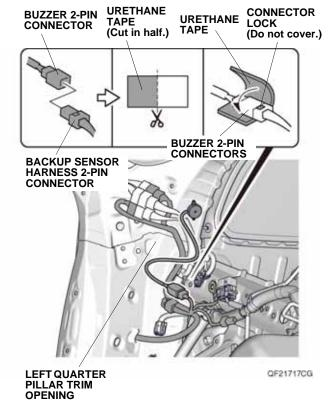
38. Using scissors, cut one urethane tape in half, and attach one half of urethane tape around the buzzer 2-pin connector.
