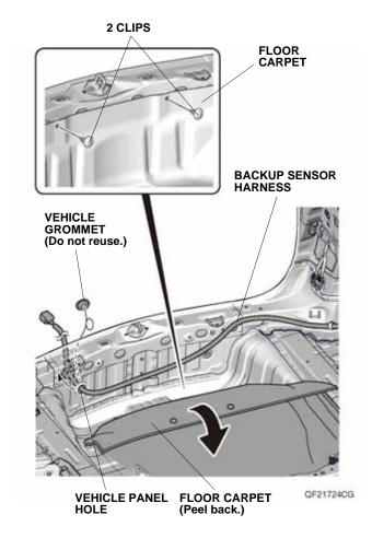
53. Secure the grommet on the backup sensor harness into the vehicle panel hole.
