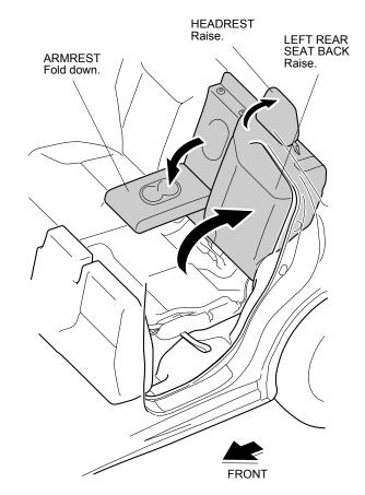
5. Install the left rear seat back cover over the left rear seat back. Insert the left rear seat back cover under the headrest guide, and insert the tab into the left rear seat back. Secure the fasteners to the left rear seat back.
