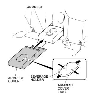
8. Raise the armrest. Pull the armrest cover between the armrest and left rear seat back, and secure the fasteners on the armrest cover as shown.
