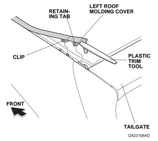
Pull the left roof molding toward the outside of vehicle to release the locking tab, and then press the locking tab toward the inside of vehicle, and release the left roof molding from the vehicle. When removing the left roof molding, start from the rear of vehicle and work towards the front.
