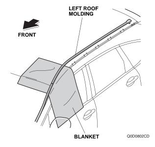
6. Place an empty cardboard box (approx. 120 mm tall) under the left roof molding near the mark.
