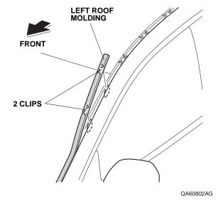
10. Insert flat-tip screwdrivers alternately between the green clip and the stud bolt as shown. While pulling on the green clip, release the locking tab on the green clip from the groove on the stud bolt notch by notch, and remove the green clip. Repeat the same procedure to remove the two purple clips.
