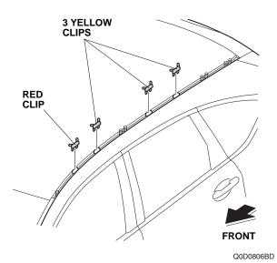
Using a flat-tip screwdriver wrapped with tape, remove the left roof molding cover from the left roof molding (one retaining tab). Discard the left roof molding.
