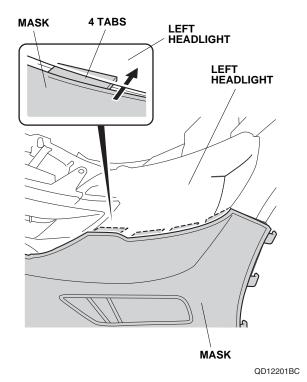
4. Attach three hooks to the inside edge of the front bumper. Repeat on the right side.
