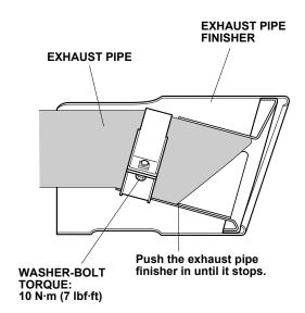
3. Start the engine, and rev it up a few times. Listen for vibration from the exhaust pipe finisher, and adjust if necessary.
