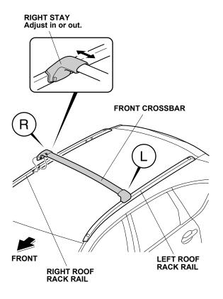
Secure the front crossbar to the roof rack rails using four bolts. Torque the bolts to 10 N·m (7.3 lbf·ft).
