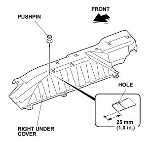
11. While wearing eye protection, drill the pierced mark on the right under cover with a 3 mm drill bit, then enlarge the hole to 10 mm using a 10 mm drill bit.
