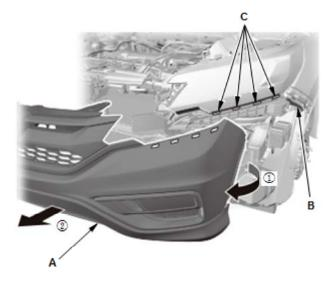
4. With the help of an assistant, while pulling the front bumps (A) away from the side spacer (B), release the bumper fro the hooks (C) on the upper beam.
