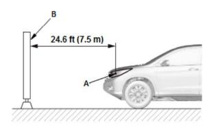
2. Park the vehicle so that the center mark of the headlight (*i* is 24.6 ft (7.5 m) away from a wall or screen (B).
