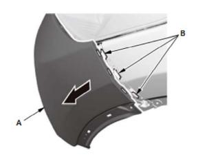
2. Pull out the front bumper (A) at the wheel arch area to release it from the hooks (B) on the side spacer.
